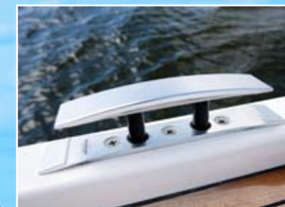
In the detail are stylish pop-up cleats (below), and teak dressing for the bowsprit and anchor winch (left).
